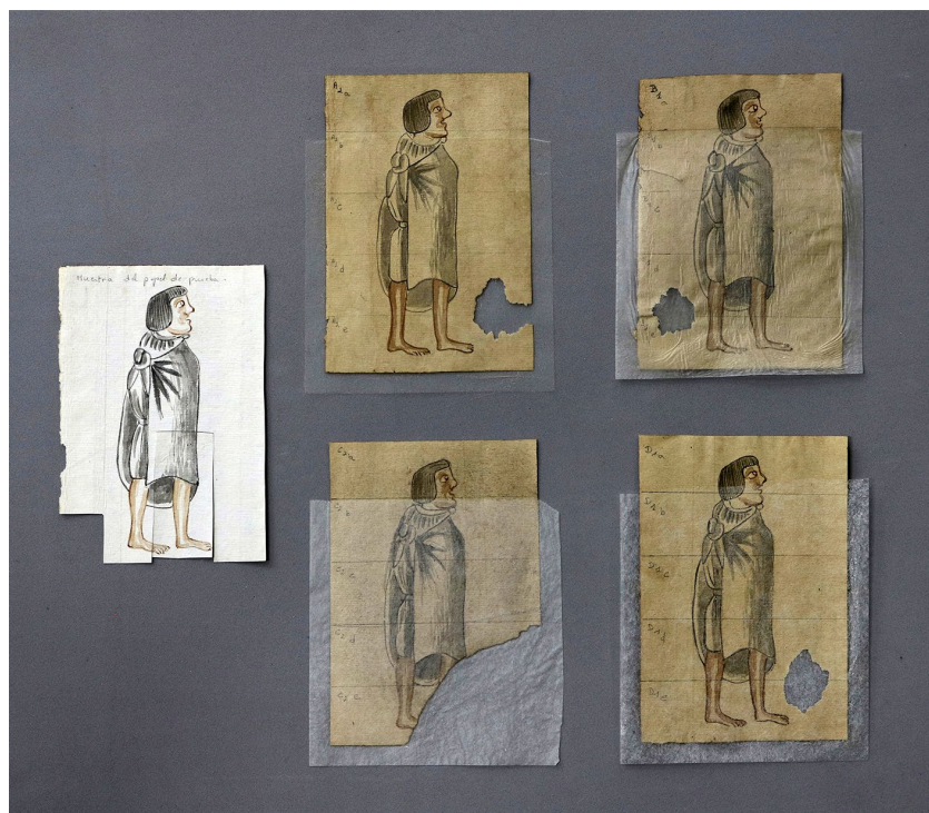
Figure 4. Tests of adhesives and lining materials for the restoration of the Yanhuitlán Codex . Image: TDG, ©CNCPC-INAH, 1993.
