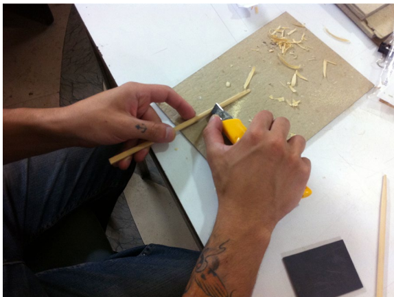
Figure 9. The construction of one's tools adapted to the needs of restoration work is part of the contents of the training that was given in various institutions. Image: ©Ana Masiello.
