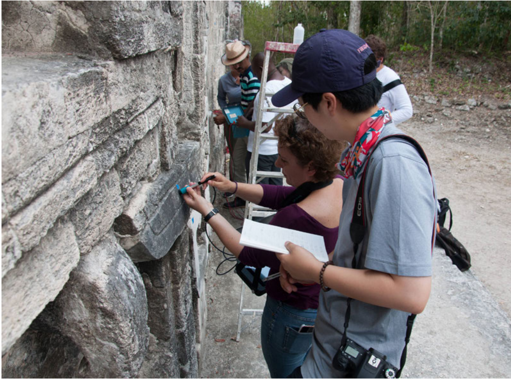
Figure 4. Students of SC17 Conducting hardness tests in structure 2 of Chicanná. Image: ©Valerie Magar.
