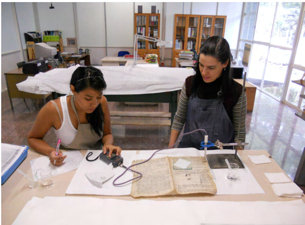
Figure 10. pH measurement with potentiometer of a work of art from San Nicolás Coatepec. Image: Archivo del Taller de Documentos Gráficos, ©CNCPC-INAH, 2012.
