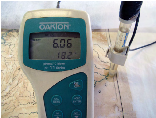
Figure 9. Measurement of the final pH of the work. Image: Martha Cárdenas, ©AGN, 2020.
