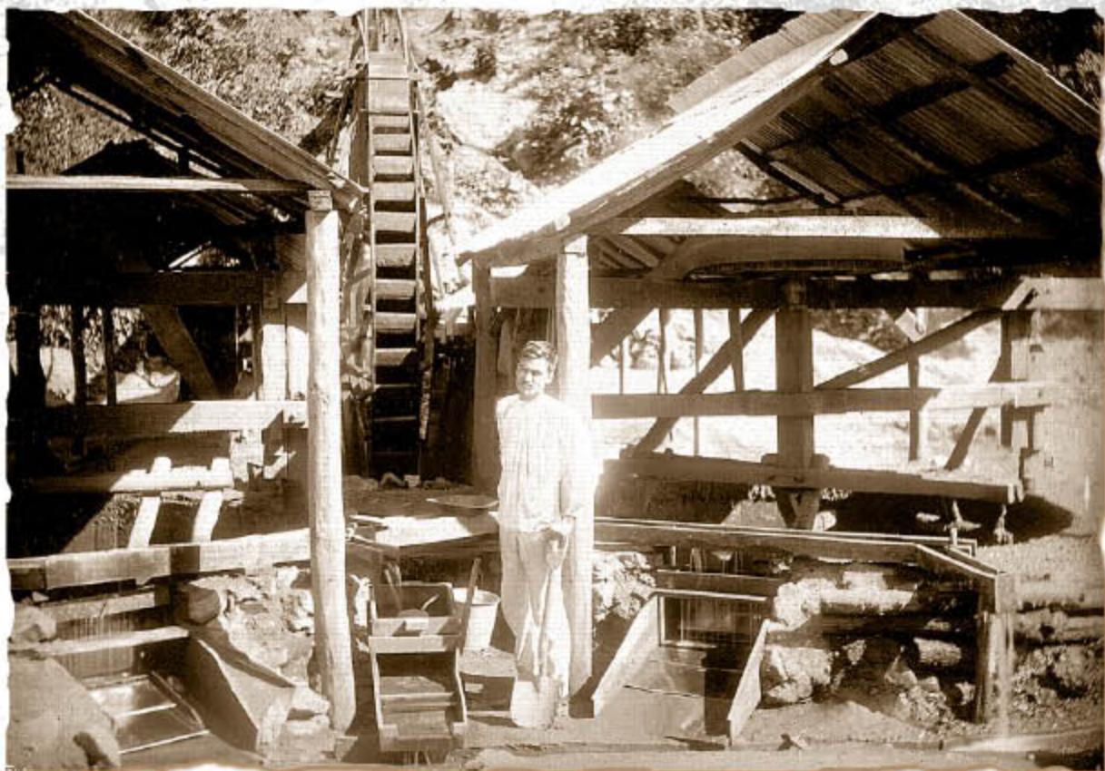
Foto 7: Instalación de canales y rueda hidráulica para lavar oro. Placeres del Oro. © Wicks, S. Robert & Harrison H. Roland, Buried Cities, Forgotten Gods. William Niven's life of discovery and revolution in Mexico and the American Southwest , Texas Tech University Press, 1999.
