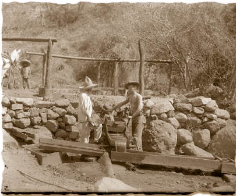
Foto 3: Cajonero y contracajonero para el lavado de oro. Placeres del Oro. © Wicks, S. Robert & Harrison H. Roland, Buried Cities, Forgotten Gods. William Niven's life of discovery and revolution in Mexico and the American Southwest , Texas Tech University Press, 1999.
