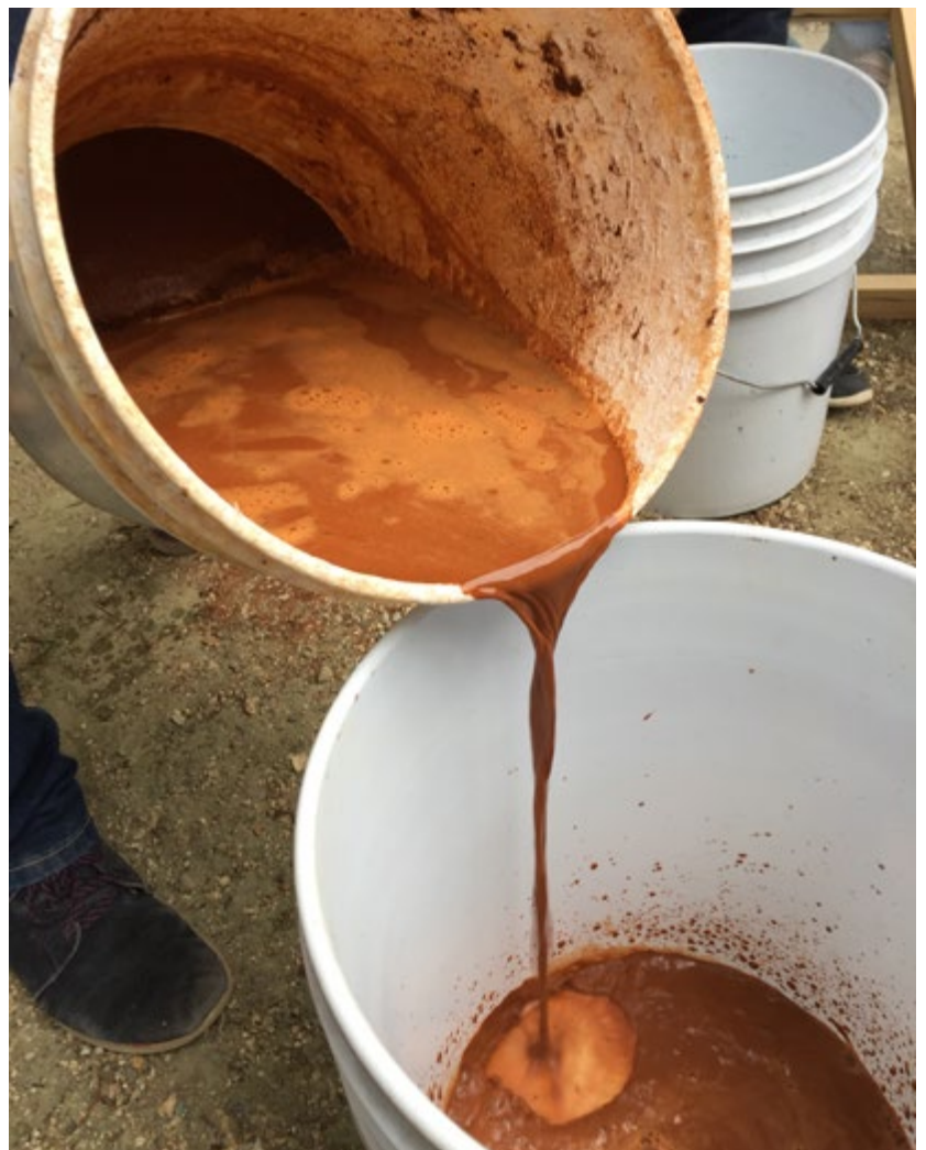
FIGURE 4. Decantation of soil to extract its clay after the silts and sands have settled to the bottom of the container (Photograph: Luis Fernando Guerrero Baca, 2018).
