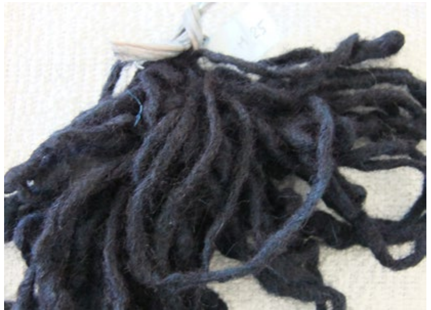
FIGURE 8. Wool dyed in the laboratory using the hydrosulfite bath method (Photograph: Sergio Franco Maass, 2017).
